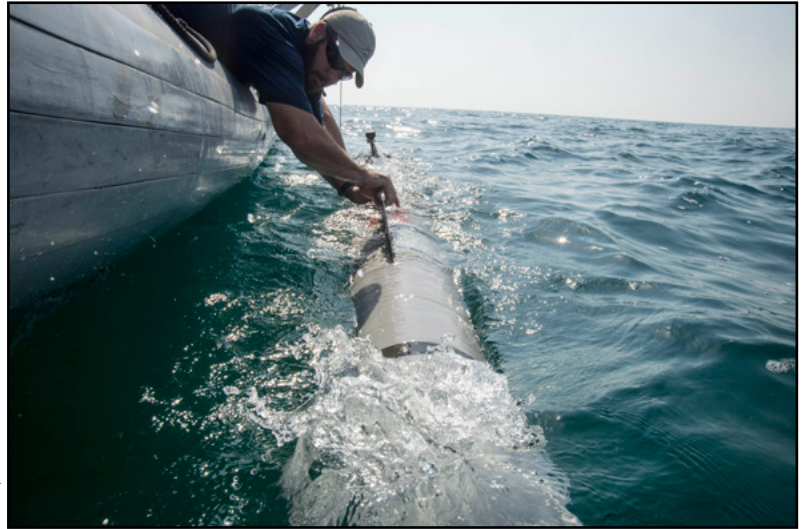
An MK18 MOD2 Unmanned Undersea Vehicle. Photo: Specialist 3rd Class Jonah Stepanik/US Navy
